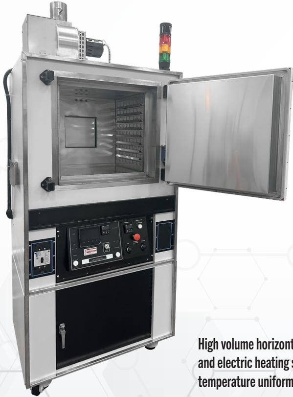
High volume horizontal air recirculation system and electric heating system allow for maximum temperature uniformity in performance
