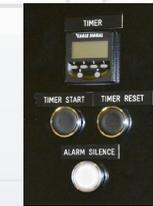
End of Process Alarm with Alarm Silence
